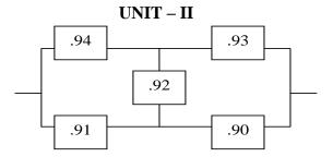
A system of independently operating elements is represented by the bridge network above. The numbers are component reliabilities. Use the delta-star transformation to compute system reliability. Verify your answer using the decomposition approach.
